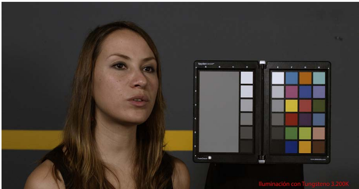
Lighting with Tungsten light to 3200. 4K DPX from RAW with S-Gamut/S-Log2
