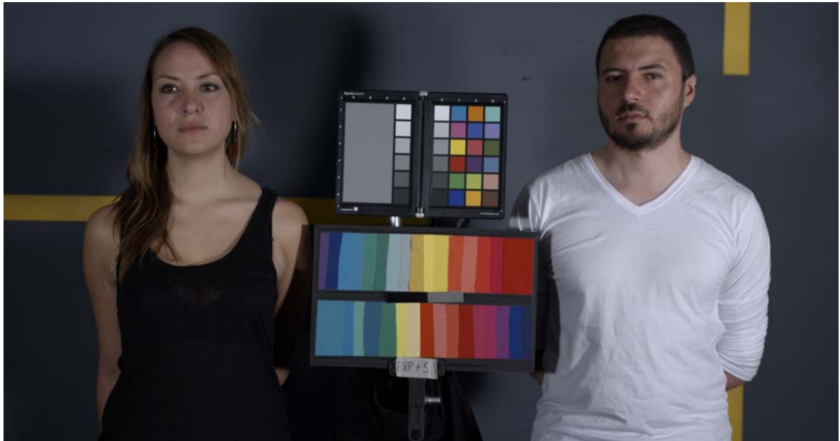
4KDPX 16 bit from RAW. Overexposed 5 stops regarding the base exposition and graded to the neutral gray.
