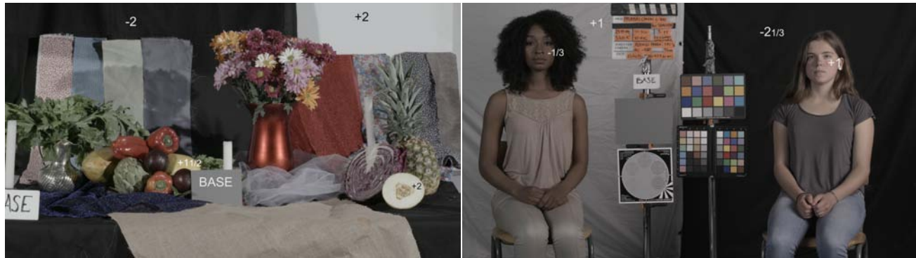
T stops values of reflected light in reference to the Mid Gray 18%
