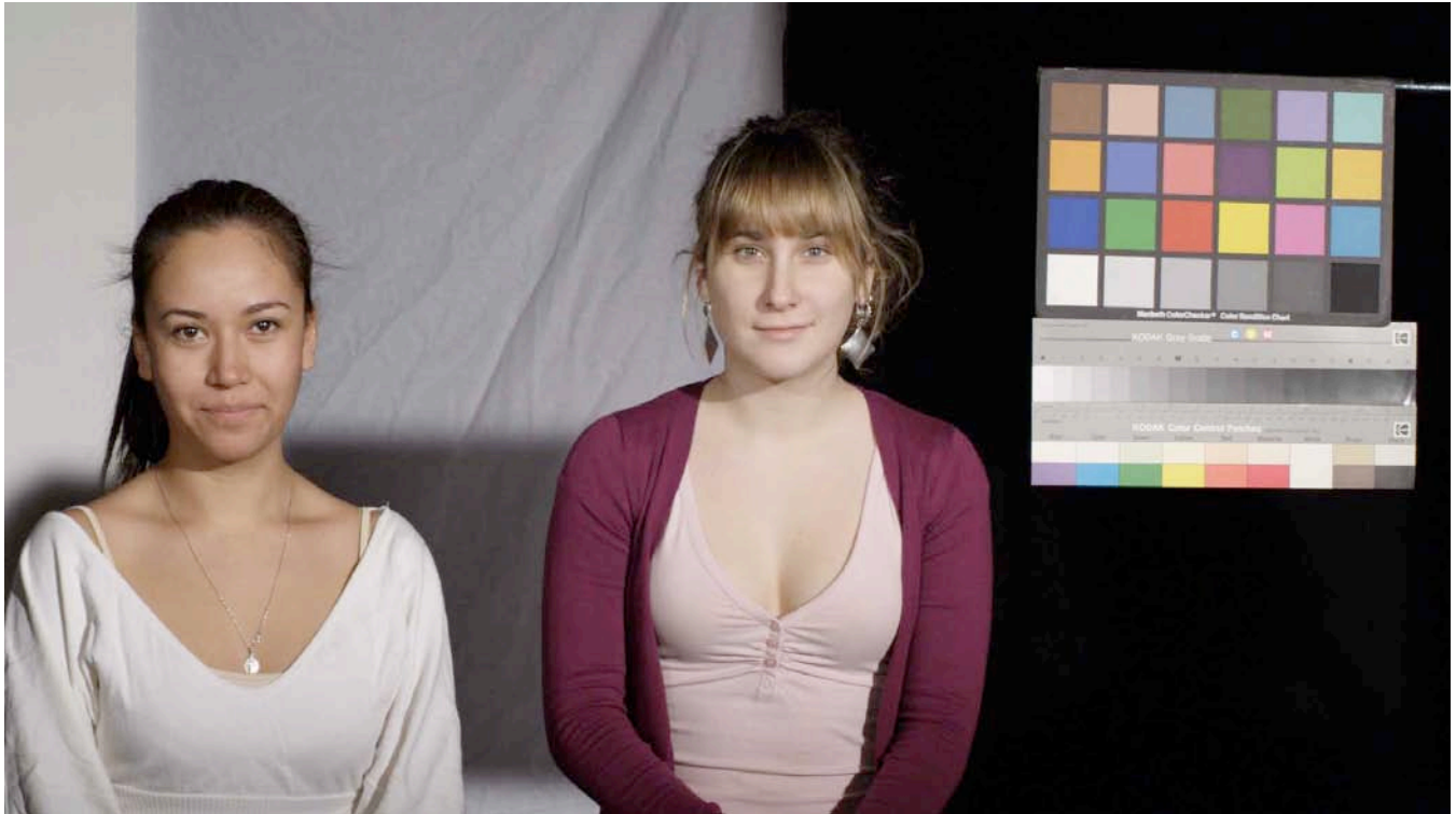
Curva Slog Rango extended Preset 3200°K F 50mm T 9.6. Etalonada
