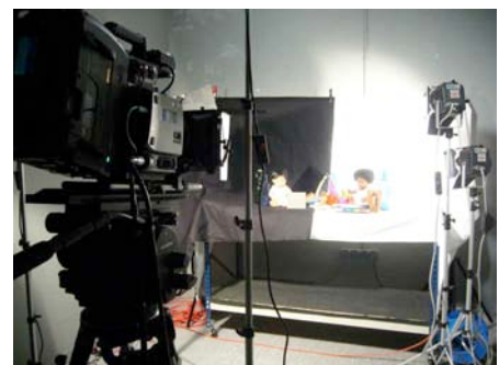
Curva S-Log DR extended. Preset 5.600°K F 24mm T6.8 Filtro Pola+ND1.2.Detail -60. Etalonado
