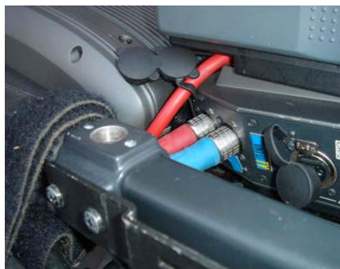
The handle in L hinders the connection Dual Link
