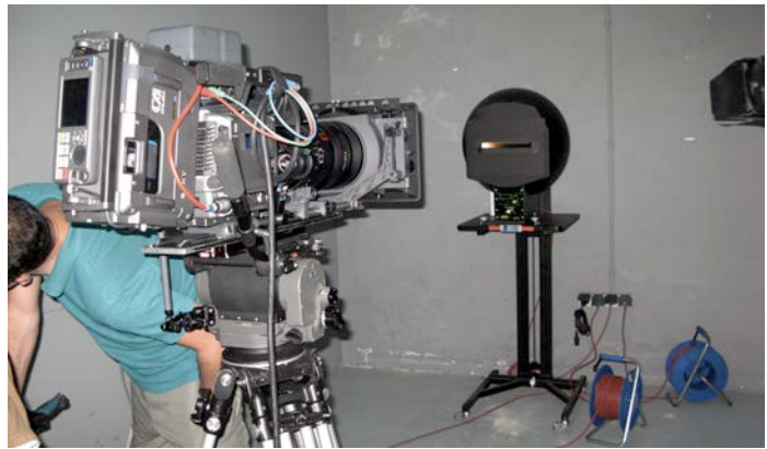
Images of the test room at Info Tv during a still life shot where we can see the different configurations of the camera. Also shooting the Stouffer Transmission Step Wedge mounted on a light sphere. In the picture, Ramiro Sabell, First Assistant Camera.
