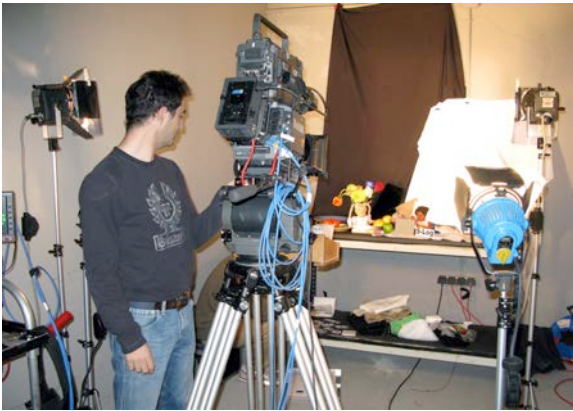
Images of the test room at Info Tv during a still life shot where we can see the different configurations of the camera. Also shooting the Stouffer Transmission Step Wedge mounted on a light sphere. In the picture, Ramiro Sabell, First Assistant Camera.
