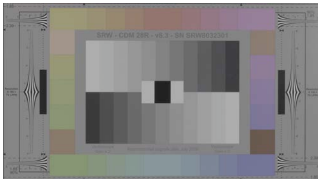
Observe in this chart with S - log gamma, the minor luminosity of the half grays and the high lights. Note: The values in the waveform are in %
